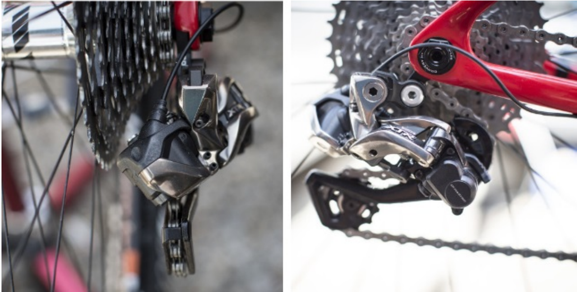
Joonis 2. Pildil on Shimano XTR Di2. Cunningham, R. (30.05.2014). First Look: Shimano XTR Di2 Electric Shifting. Kasutamise kuupäev 20.09.2014., allikas: http://www.pinkbike.com/news/first-look-shimano-xtr-di2-electric-shifting.html .
