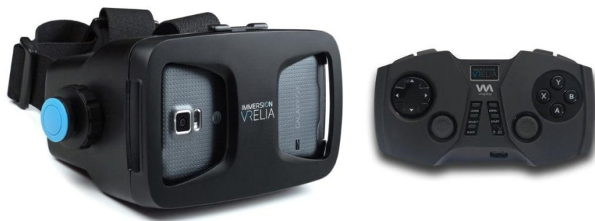
Figure 3.. ImmersiON-VRelia GO HMD and gamepad controller 1 .
