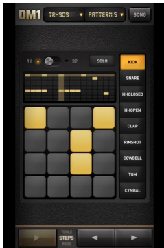
Figure 11. The iPhone version of the DM1 breaks the 16 step grid into 4 x 4 rows.
