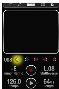
Figure 7. The interface of Korg iKaossilator 17 with no visible separation points of the XY touch area.
