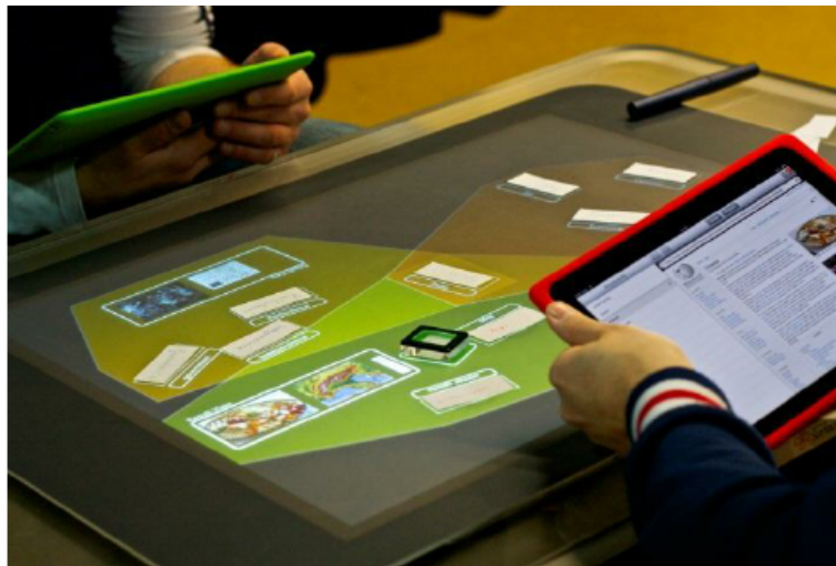
Figure 2.1: TwisterSearch: DUI supporting collaborative web search (Rädle et al., 2013)
